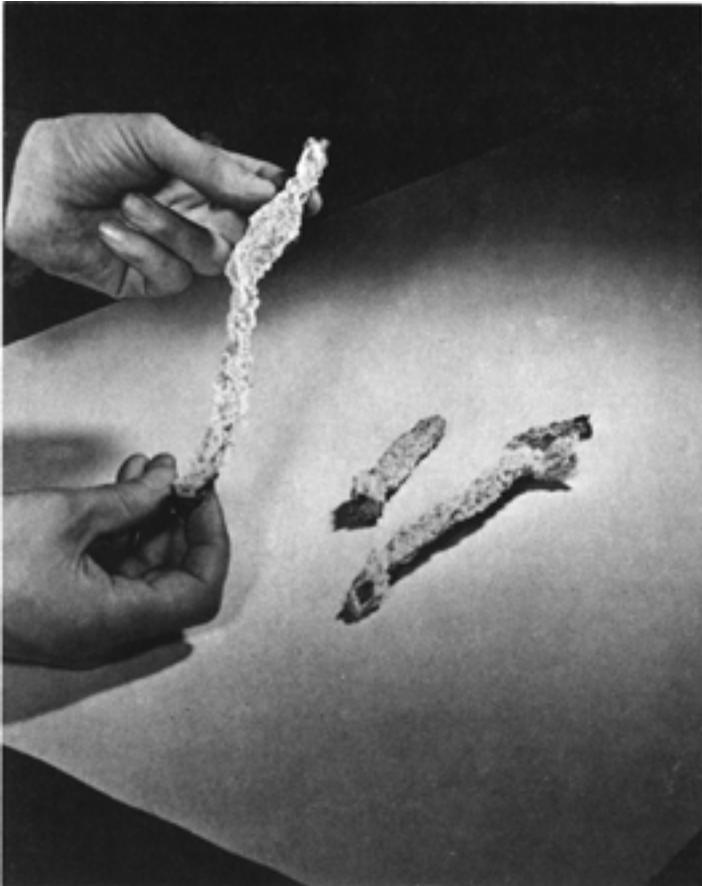
Figure 10.4: Artificial fulgurites produced by P. L. Bellaschi, Westing house Electric Corporation, by allowing an electrical discharge to pass through quartz sand. The hollow tubes of solidified sand are close replicas of natural fulgurites.
