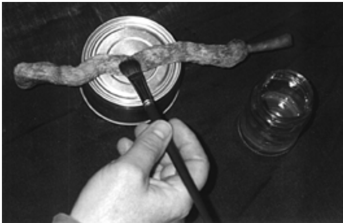
Russ McCarty paints on a layer of hardener to stabilize the fulgurite for moldmaking.
